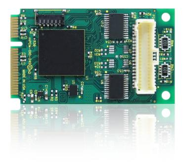
New Line of Rugged PCI Express Mini Cards for Easy and Flexible Digital I/O Expansion
