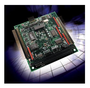
New 12-Channel Analog I/O Board for PC/104 Offers More Flexible Depopulation Options, Digital Change-of-State Detection and Lower Cost than Most Boards at its Price Point
