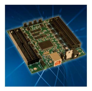
High-Speed USB 2.0 Module Provides 96 or 48 Lines of Optimized Digital I/O for Flexible and Economic Digital Control and Monitoring
