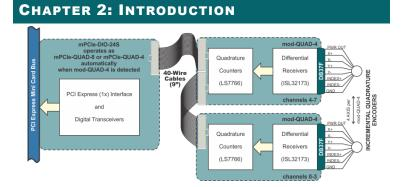
PCI Express Mini Card (mPCIe), a low-profile small-footprint bus standard originally intended for adding peripherals to notebook computers, has become the de-facto standard for highperformance, small form-factor devices in many applications.
