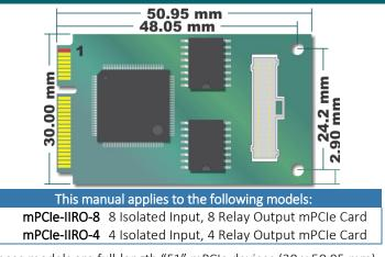
These models are full-length "F1" mPCIe devices ( $30 \times 50.95$  mm), and include a required 9" (229mm) 40-conductor cable connected to a panel-mountable DB-37M Isolation Module. The Isolation Module is Mobile-ITX sized ( $1.772'' \times 2.952''$ ) for broad installation compatibility. All units are RoHS compliant.
