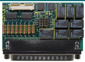
The Isolation Module includes jumpers to enable input filters with a 4.7ms time-constant, optimized for dealing with AC signals, but useful for a wide variety of transient-mitigation tasks.
