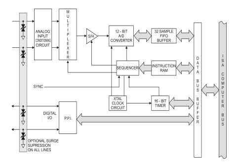
Figure 1-1: PAD128 Block Diagram
