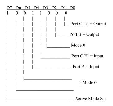
This corresponds to 98 hex. If the card base address is 2D0 hex, use the C command to write to the control register as follows:
