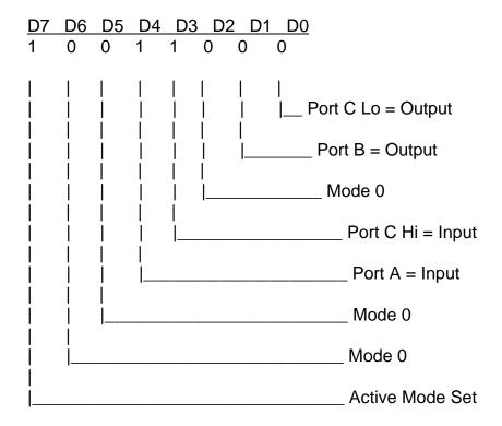
This corresponds to 98 hex. If the card base address is 2D0 hex, use the C command to write to the control register as follows:
