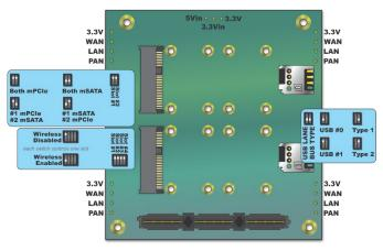
The 104e-mPCle-4 modules need the following configurations:
